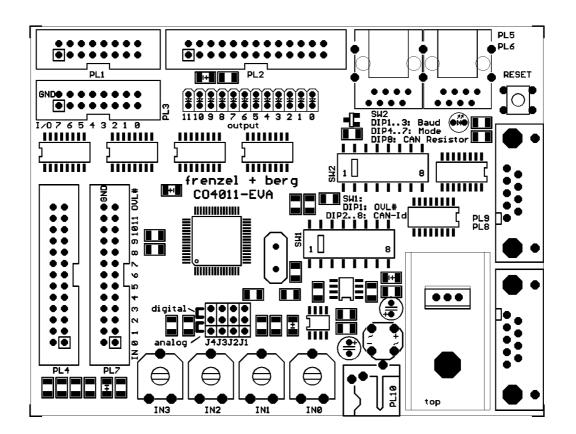
PL1, PL2 and PL4 are implemented, to connected the input/output port bits to an application hardware using simple flat cable. PL3 and PL7 may be used to place any jumpers for activation of input bits. Note that jumpers must not be set at connector PL3 if I/O lines IO0 to IO7 are configured as output bits.
