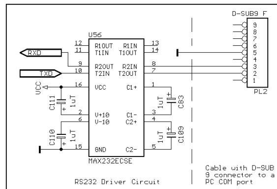
(Such a circuit is also needed with the FLASHJET programming tool)
